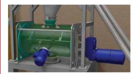
Mixer is a device designated to mix dry products placed in the mixing chamber and in effect creating a homogenous mixture.
