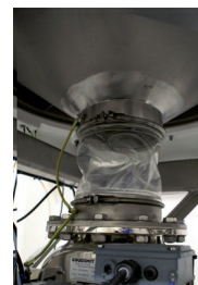
Flexible connections in the JACOB assembly system
